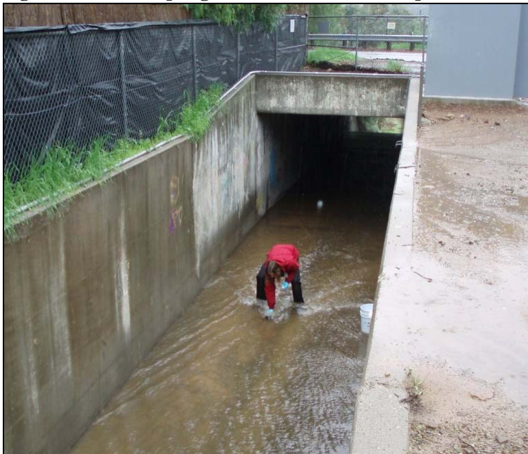
Figure 6. Grab Sampling at Mid-Stream, Mid-Depth
