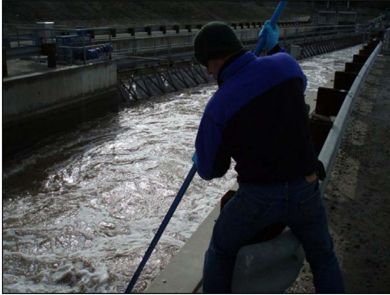
Figure 7. Grab Sampling Using Extended-Reach Swing Sampler
